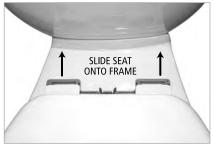
5. Slide seat onto hinge until the red locking clips click outwards. If position is incorrect, press the red locking clips towards the centre, remove seat, loosen bolts and slide the frame on the supports to the desired position before retightening.
